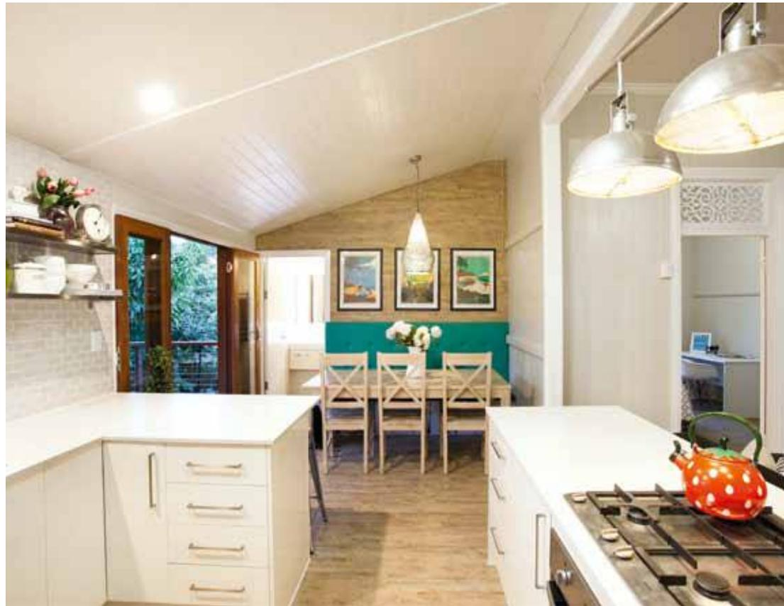
**Above and below** VJ boards from the removed walls were reused to line the ceiling of the new dining area. A banquette/dining booth was built against the new bathroom wall, allowing the dining table to be tucked closer to the wall, freeing up space
